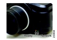
The PVC2300 and WVC2300 cameras have two LEDs to let you know how the camera is functioning.
