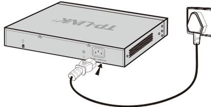
Figure 4-3 Connecting to Power Supply
