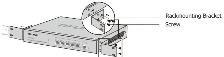
Figure 2-2 Bracket Installation
