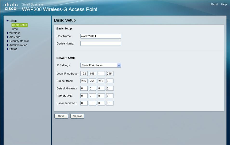
The screenshot shows the Cisco WAP200 Wireless-G Access Point configuration interface. The title bar reads "Small Business WAP200 Wireless-G Access Point" with "About Help" on the right. A left-hand navigation pane lists "Setup" with sub-items: "Basic Setup" (highlighted), "Time", "Wireless", "AP Mode", "Security Monitor", "Administration", and "Status". The main content area is titled "Basic Setup" and is divided into two sections: "Basic Setup" and "Network Setup".
