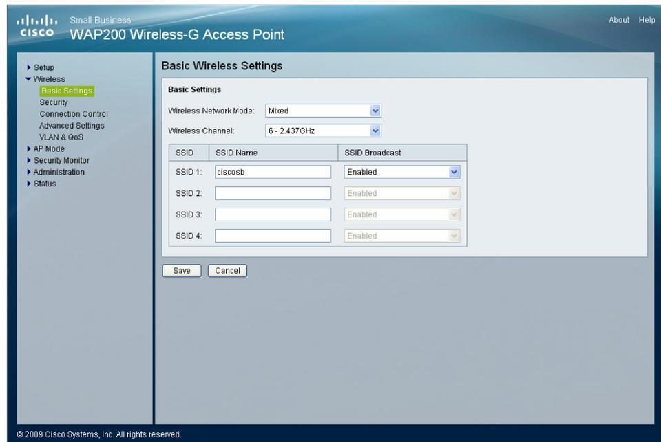
To configure the Wireless Network basic attributes for the entire system and for each SSID, follow these steps:
