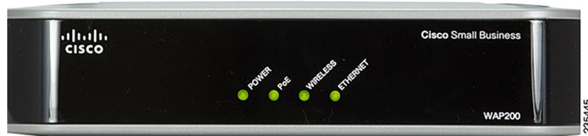
**Power LED**—Lights up and remains lit when the access point is powered on.
