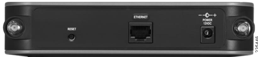
**Reset Button**—There are two ways to reset the access point's factory default configuration:
