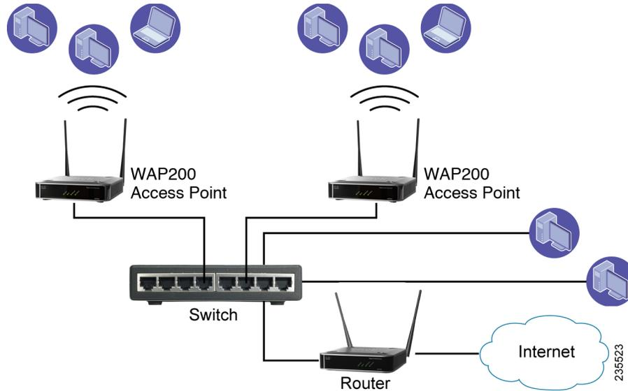
In this example, the wireless access points connect to and receive power from a PoE Cisco switch. Each access point can connect multiple wireless devices to the network.
