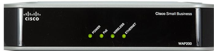
**POWER LED**—(Green) Lights up and remains lit when the access point is powered on.
