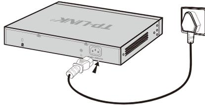
Figure 4-3 Connecting to Power Supply
