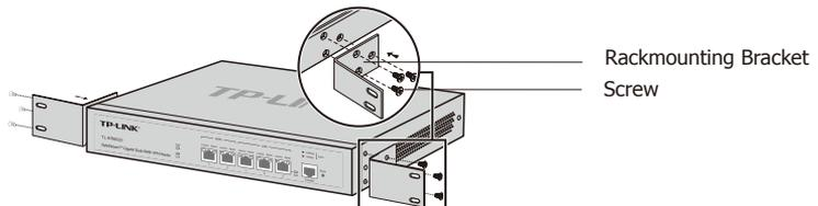
Figure 2-2 Bracket Installation
