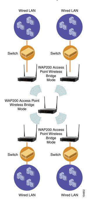
For the Wireless Repeater and Wireless Bridge modes, the Wireless Network mode, Channel, and Security settings must be the same for other remote wireless access points and devices.
