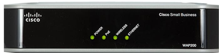
**POWER LED**—(Green) Lights up and remains lit when the access point is powered on.
