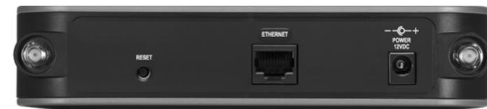
**RESET Button**—Resets the access point to the factory default configuration. You need to press this button for about ten seconds to reset the access point.
