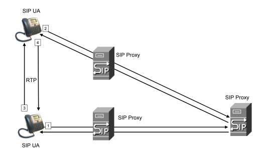
SIP message routing is dynamic. If a SIP proxy receives a request from a UAS for a connection but cannot locate the UAC, the proxy forwards the message to another SIP proxy in the network. When the UAC is located, the response is routed back to the UAS, and a direct peer-to-peer session is established between the two UAs. Voice traffic is transmitted between UAs over dynamically-assigned ports using Real-time Protocol (RTP).
